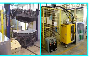
**RTM**: Uniconform® is suitable for low to medium complexity shapes and it allows to reach high glass content (up to 55%).
